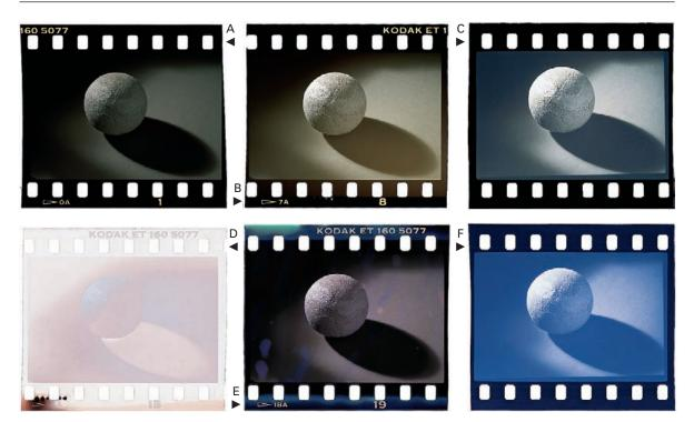
**Figure 11.32** Some E-6 colour slide processing faults. A is correctly processed. B: fogged to low-level light before processing. C and D: fogged during processing. E: contamination of first developer with fixer (including fix spots). F: colour developer contaminated with bleach
