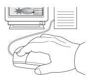
**Figure 14.3** Mouse. Shifting the whole mouse moves the cursor (arrow here) anywhere on screen. Single or double clicking a button calls up whatever tool, command bar icon, etc., the cursor has been positioned over. See Figure 14.11
