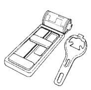
Figure 11.6 35 mm tools. Left: film retriever, inserted into a 35 mm cassette in daylight, pulls out the tip of exposed film which has been wound in. Right: opener to remove the end of the cassette, in darkness
