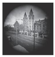
**Figure 5.11** Lens coverage. The total circular image patch formed by an 85 mm lens designed to cover 35 mm format (inner frame). Used as a normal angle lens on a  $6 \times 6$  cm format camera edges begin to darken. And attempting to use it as a wide-angle on  $4 \times 5$  in (outer frame lines) uneven illumination and corner 'cut off' becomes obvious, particularly when the lens is stopped down. See also Camera movements, page 306
