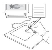
**Figure 14.4** Graphics palette. Together with its cordless pen this serves the same functions as the mouse. It makes it easier to trace around a complicated shape, draw freehand or sign your name. A small switch on the pen provides the equivalents of mouse clicks
