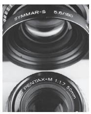
**Figure 3.3** Engraving around lenses here shows (top) name of lens; maximum aperture *f*/5.6 and focal length 180 mm and (bottom) name, *f*/1.7 maximum aperture, 50 mm focal length
